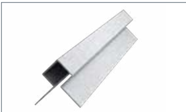
4. Swisspearl External Corner Large 32x20x26mm coloured aluminium profile for 90° angle
